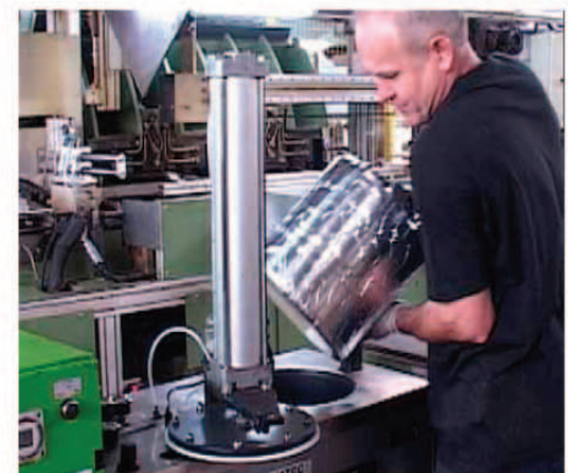
Inserting a new bag or "slug" of adhesive into the melt unit
